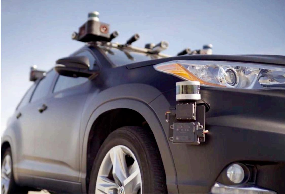
Building a fully autonomous vehicle requires a significantly more robust suite of sensors than cars with advanced driver assist features have today. There are no shortcuts to building a best-in-class, next-generation sensor suite for our vehicles.
